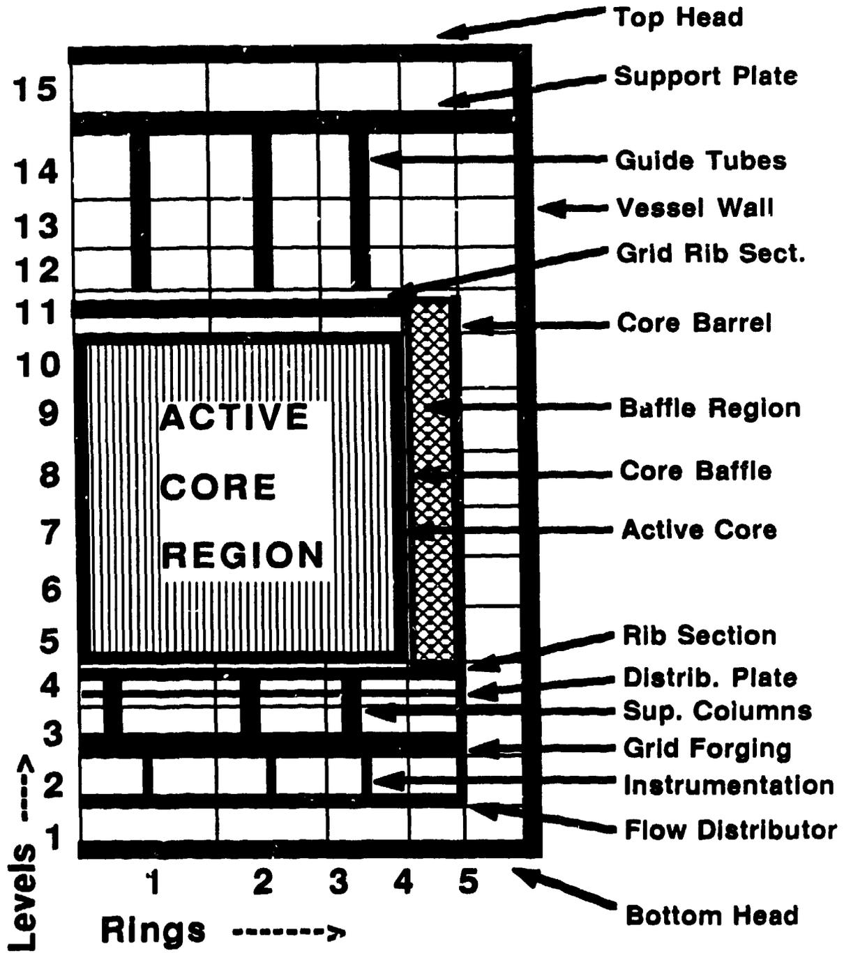
Figure 2. TMI-2 TRAC PRIMARY-SYSTEM MODEL
